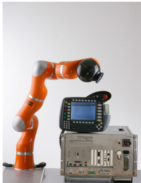
Figure 1: KUKA Lightweight Robot (LWR) with KUKA Robot Controller (KRC 2r) and KUKA Control Panel (KCP).
