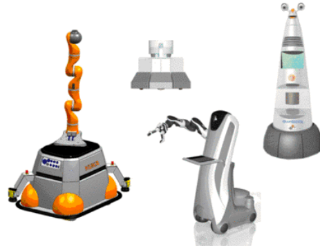
Figure 2: Overview of some of the possible Robotics RTD Platforms (RRPs) to be used in the project (from left to right): KUKA omniRob, mobile base of BlueBotics, IPA Care-O-Bot, BlueBotics Gilberto.
