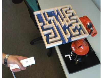
KUKA youBot arm and labyrinth – remotely controlled by Nintendo Wii controller © University of Augsburg Software Engineering
