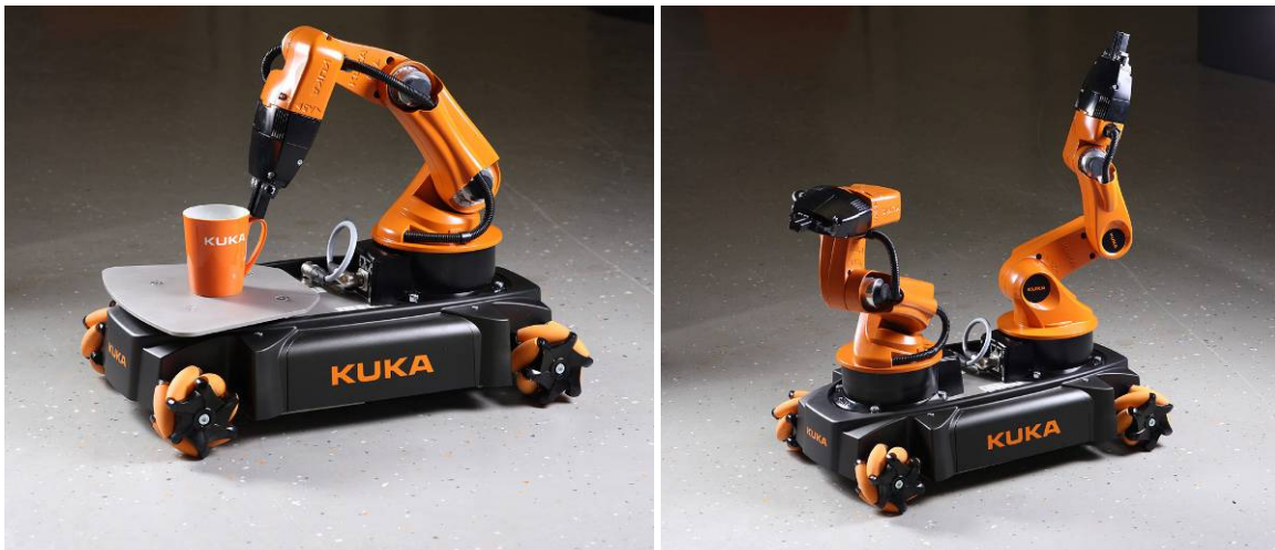
Figure 21: The youBot in a one- and a two arm configuration
