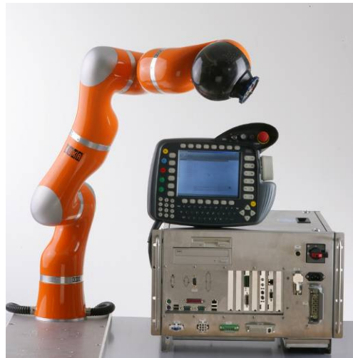
Figure 10: The KUKA lightweight robot with KRC2 Ir controller
