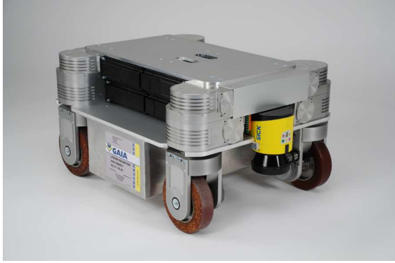
Figure 1: Mobile Base of Care-O-bot® 3
