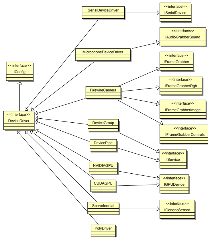
Figure 4.7: YARP Hardware Abstraction Hierarchy
