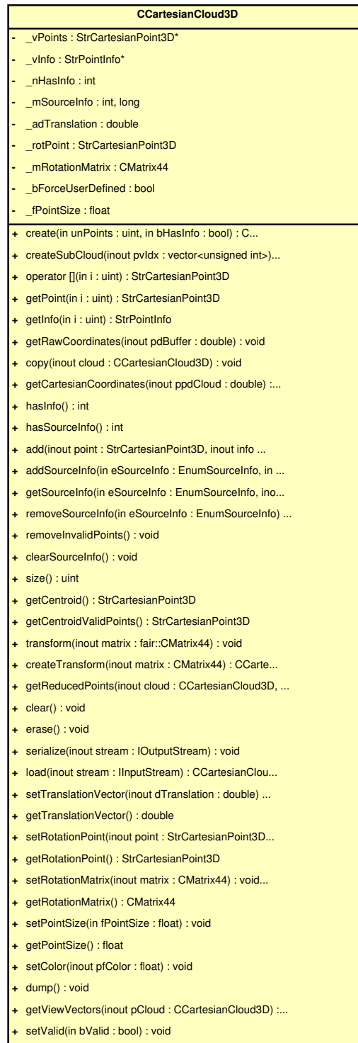
Figure A.12: UML class diagram of Cartesian point cloud representation in FAIR library.
